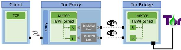
**Fig. 12.** Testbed deployed, with two wireless networks connecting the client (Tor proxy) and the Tor bridge.
