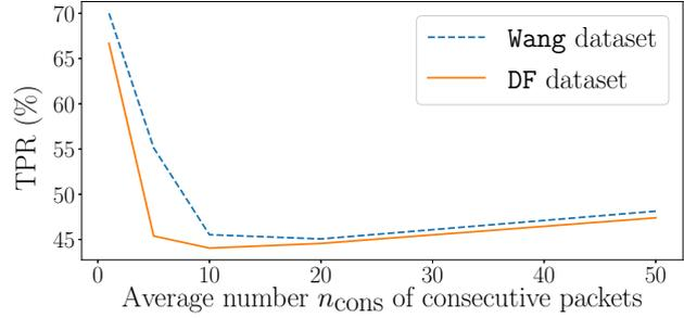
**Fig. 17.** Performance of the DF attack on traces protected with the splitting scheme described in Section 5.4, for different values of the average number of consecutive packets  $n_{\text{cons}}$  and a geometric distribution. Closed-world experiment, Wang and DF datasets,  $n_{\text{pr}} = 300,000$ .
