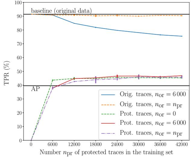
**Fig. 3.** Performance of the attack on original traces and traces protected with the splitting scheme described in Section 5.3, for different sizes of the training set. Closed-world experiment, Wang dataset,  $n_{cons} = 1$ .
