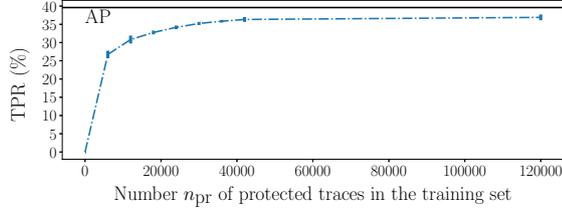
**Fig. 5.** Performance of the  $k$ -fingerprinting attack against HyWF, for different sizes of the training set. Closed-world experiment, Wang dataset.
