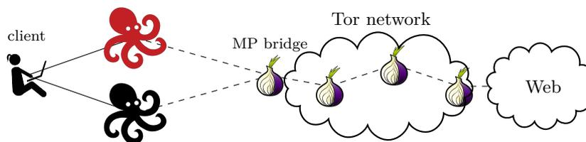
**Fig. 2.** Model where the client is multihomed, with two different adversaries, and connects to a multipath-compatible Tor bridge (MP bridge), typically located in another country.
