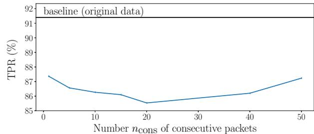
**Fig. 13.** Performance of the  $k$ -fingerprinting attack on traces protected with a round-robin scheme, for different values of the number of consecutive packets  $n_{\text{cons}}$ . Closed-world experiment, Wang dataset.
