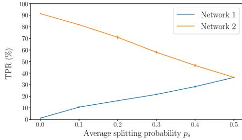
**Fig. 11.** Performance of the  $k$ -fingerprinting attack when the client sends a fraction  $p_s$  of its traffic through Network 1, for different values of  $p_s$ . Closed-world experiment, Wang dataset.
