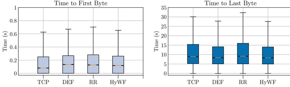
**Fig. 9.** Box-and-whisker plots of the TTFB (left) and TTLB (right) for single-path TCP (TCP) and different configurations of MPTCP: default scheduler (DEF), round-robin (RR) and our proposal (HyWF). *exp* dataset with 10,000 traces per scenario.
