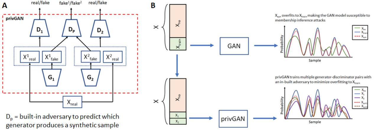
**Fig. 1.** A) The privGAN architecture with 2 generator-discriminator pairs. B) Illustration of how privGAN provides protection against membership inference attacks by preventing memorization of the training set.
