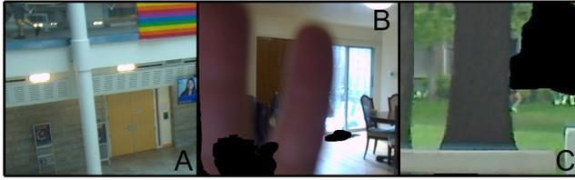
**Figure 12: Common failure situations. (A) Thermal masking is prevented by glass blocking the transmission of infrared waves. (B) Imperfect camera alignment reveals fingers that are directly touching the RGB camera. (C) Pixel resolution masking limitations resulting in PII leakage.**
