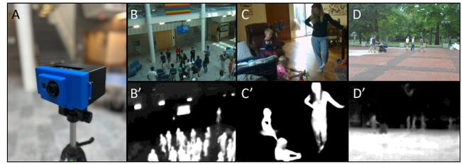
**Figure 6: Image of the PrivacyLens prototype in a tripod-mounted 3D-printed enclosure (A), images from the deployment study showing the office atrium (B), home living room (C), and public park square (D). The thermal camera’s images have been contrast-enhanced for ease of viewing.**
